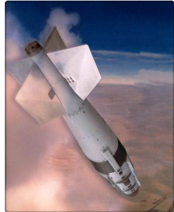
U.S. Joint Direct Attack Munitions (JDAM) - “smart bombs” use neodymium-iron-boron magnets to control the drop direction when dropped from an aircraft.
